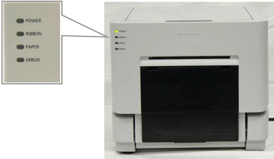
The flashing LED indicates the printer status
